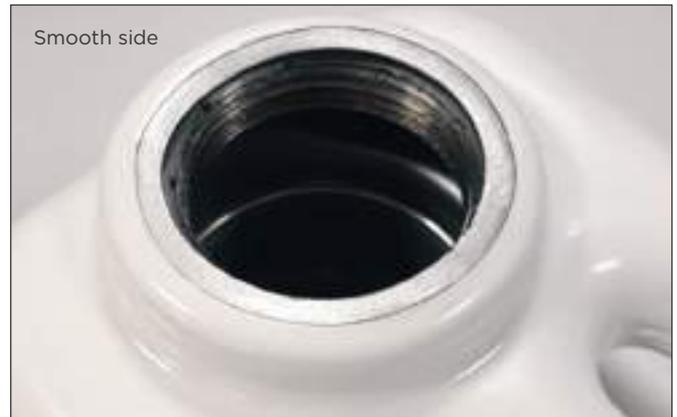
The inner surface of the nipple can be serrated or smooth. To join radiators, it is necessary to associate a serrated connection of the radiator to a serrated side of the nipple.
